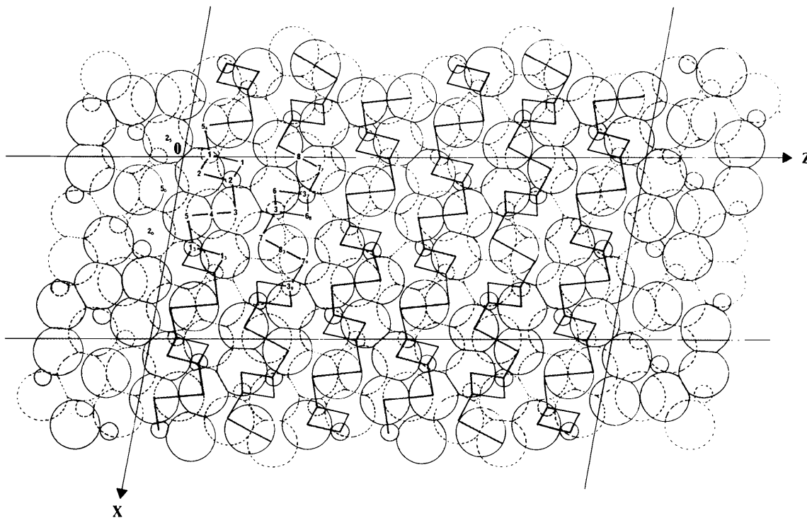
Fig. 1. \text{In}_2\text{Te}_5(\text{II}) . A projection of the structure down b showing the method of bonding. The atoms are scaled to the respective ionic radii of \text{In}^{3+} (0.81 Å) and \text{Te}^{2-} (2.22 Å). Shaded and non-shaded atoms lie near y = \frac{1}{2} and 0 respectively.
